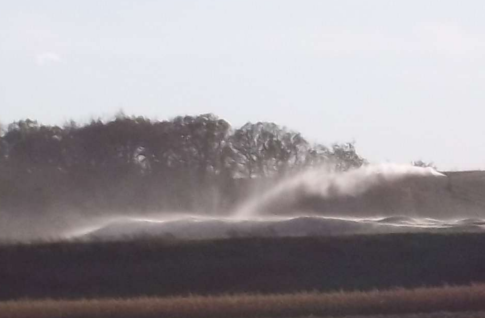
6-2011 -- The Fairmount Mine in Menomonie has two high-capacity wells for ing down sand to keep it from blowing around.
